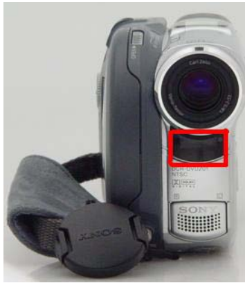
Fig. 11. Camcorder (Sony DCR-DVD201) with an integrated infrared illuminator.
